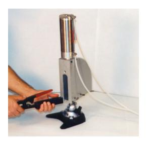
5. Position the hand tool into the bottom center channel of the Power Crimper with the moving half of the crimp tool handle facing up towards the roller above it. Make sure you insert the hand tool far enough into the channel so the ratchet of the hand tool goes through its complete re-opening cycle and allows the crimp jaws to fully open.
