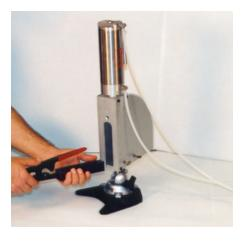
9. Insert the hand tool into its adapter, which is polarized to accept the tool.
