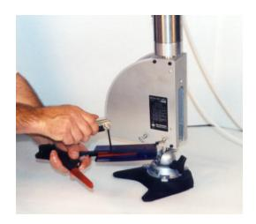
10. Tighten the Allen set screws evenly from both sides of adapter against the tool handle to hold tool securely. Over tightening set screws may distort the adapter, making it difficult to slide into tool channel. Upon completion of this step, follow
