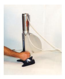
6. Equally tighten the thumbscrews provided on both sides of the channel to securely seat the tool. Do not over tighten as excessive thumbscrew pressure may distort the tool frame, preventing the tool from functioning properly.
