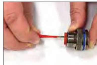
Plastic tool with contact in proper position.
