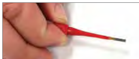
Plastic tool with contact in proper position.
