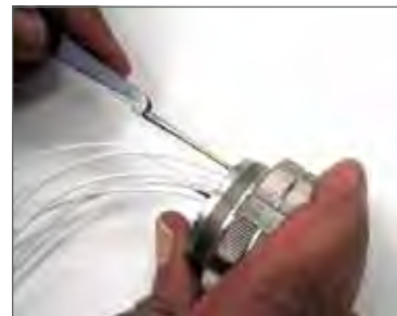
Removal of contacts with metal tool.
