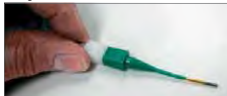
Plastic tool with contact in proper position.
