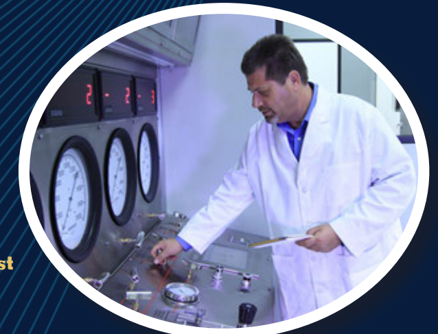
SeaKing™ and SuperG55™ QUALIFICATION TESTING: Both Glenair Series 70 SeaKing and SuperG55 rugged dry-mate subsea connectors have been tested and qualified to their 10K psi pressure rating—open-face and mated—in Glenair's state-of-the-art hydrostatic test lab. Additional testing included mating cycles, salt spray, and electrical continuity.
