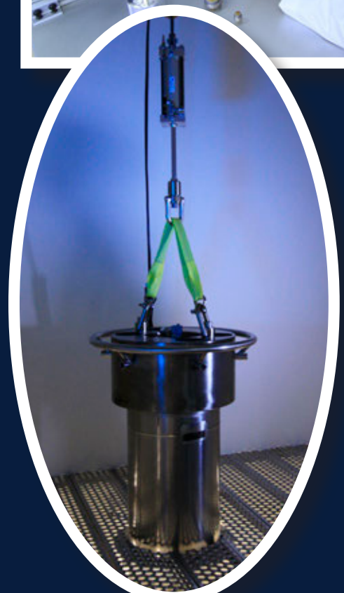
LARGE PRESSURE VESSELS: Built to accommodate complete cable assemblies, mated connectors, and customer-supplied subassemblies
