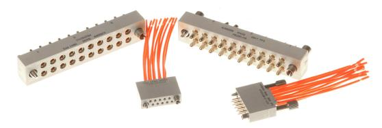
**W-Series** is the benchmark against which so many others are measured. The W-Series products are internationally accepted and approved to MIL-DTL-55302 standard. The size of this product ranges from 3 to 208 contacts and allows for a range of termination styles. The contact spacing is 0.100" (2.54 mm). Other contact options include dip solder, solder cup, right angle, flex circuit and wire wrap.
