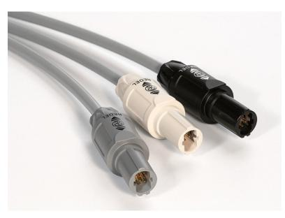
LEMO REDEL SP Connectors plastic, self-latching push-pull with an ergonomic grip, color-coding and keying options, high contact density, and an IP50 seal. They also exhibit high resistance to chemicals, shock, and sterilization processes.
